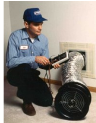
Photo of Man Conducting Duct Blaster Test:
