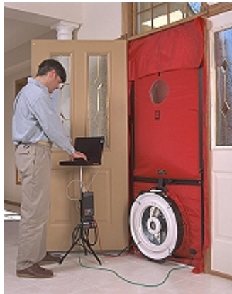
Photo of Man Conducting Blower Door Test:
